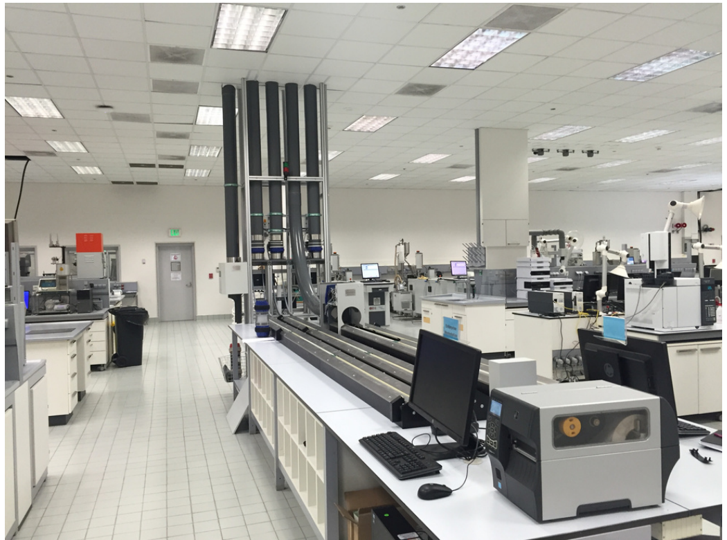
Insight into a laboratory with receiving stations with conveyor belt
