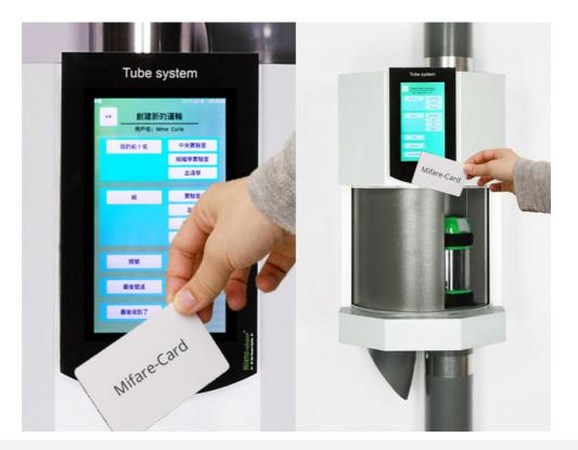
*Identification of an employee at a pneumatic tube station with MiFare reader. In addition to stations with the 10 inch touch screen, other stations can also be equipped with the MiFare reader.*
