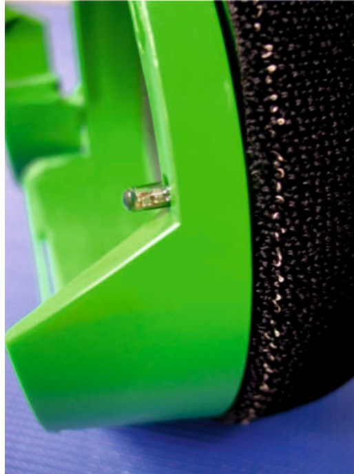
RFID tag installed in carrier
