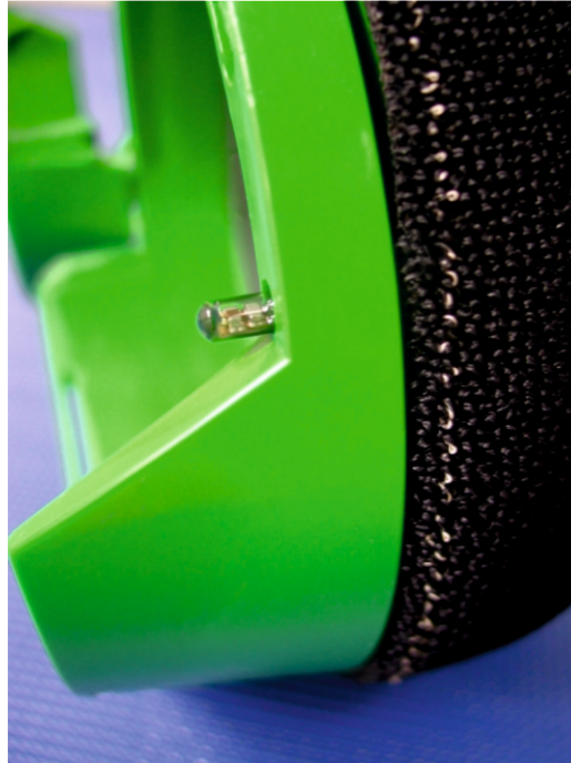
RFID tag installed in carrier
